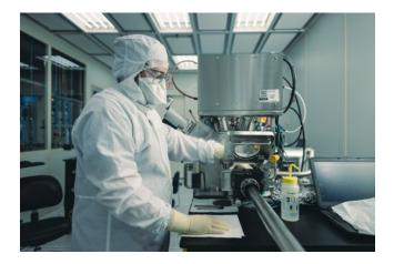
In addition to wet etching chemical hoods available inside and outside the Scifres cleanroom, there are many dry etching tools within the cleanroom for reactive ion etching (RIE), deep reactive ion etching (DRIE), asher, ion milling and vapor phase etch with a wide variety of chemistries available.
